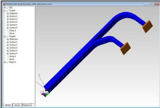
**Figure 3: Post-Optimization Light Pipe Design**
