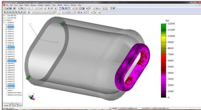
**Figure 1:** 3D Illuminance Map Shown on Light Pipe Output Surface
